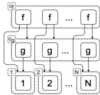
An example e-graph. Each solid box denotes an e-node and each dashed box denotes an e-class, which represents a set of equivalent terms. Labels at top-left corner denotes the e-class id. Represented terms include  $f(1, g(1))$ ,  $f(1, g(2))$ ,  $f(2, g(1))$ , etc. ( $O(N^2)$  in total).
